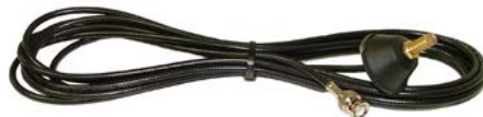
OB4.7-BNC OB-2 Base, Black, 4.7 metres RG58 low loss stranded cable, BNC male crimp connector fitted
