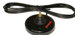
MGB-OB Magnetic OB-2 Base, steel with polished black powder coat finish, 10.5 cm diameter, heavy duty magnet, PVC matted pad on bottom, 4.7 metres RG58 low loss stranded cable side exits, no connector
