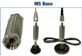
The "MS Base" medium duty stainless steel spring with 5/16"–26 TPI male and female threads will suit any mobile whip being mounted onto our OB-2 antenna bases. Screw the spring onto the base and the whip onto the spring.
