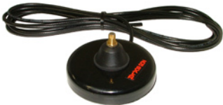
MGB-OB Magnetic OB-2 Base, steel with polished black powder coat finish, 10.5 cm diameter, heavy duty magnet, PVC matted pad on bottom, 4.7 metres RG58 low loss stranded cable side exits, no connector
